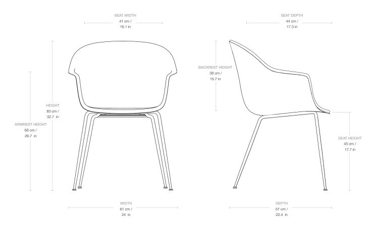
61 cm / 24 in WIDTH 57 cm / 22.4 in **DEPTH** 83 cm / 32.6 in HEIGHT SEAT WIDTH 41 cm / 16 in SEAT DEPTH 44 cm / 17.3 in SEAT HEIGHT 45 cm / 17.7 in 38 cm / 15 in **BACKREST HEIGHT** 68 cm / 26.7 in ARMREST HEIGHT
